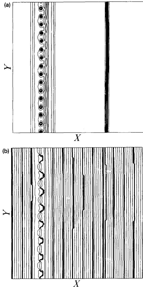
Fig. 1. Level lines of amplitude (a) and phase (b) of an established field distribution for  $\beta=2$ ,  $\alpha=0.2$  and  $T=10^4$ . A regular distribution of the spirals demonstrates the effect of spatial self-organization under random initial conditions.
